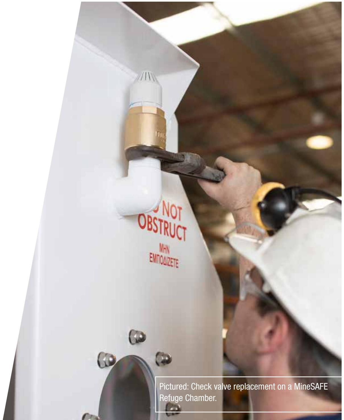
Pictured: Check valve replacement on a MineSAFE Refuge Chamber.
